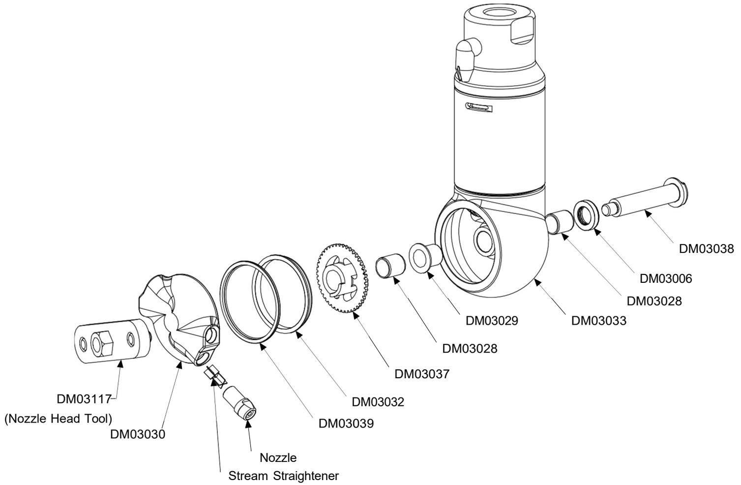
Figure 4: Nozzle head disassembly.
