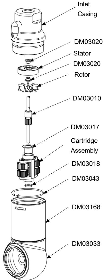
Figure 12: Body shell and inlet casing assembly.
