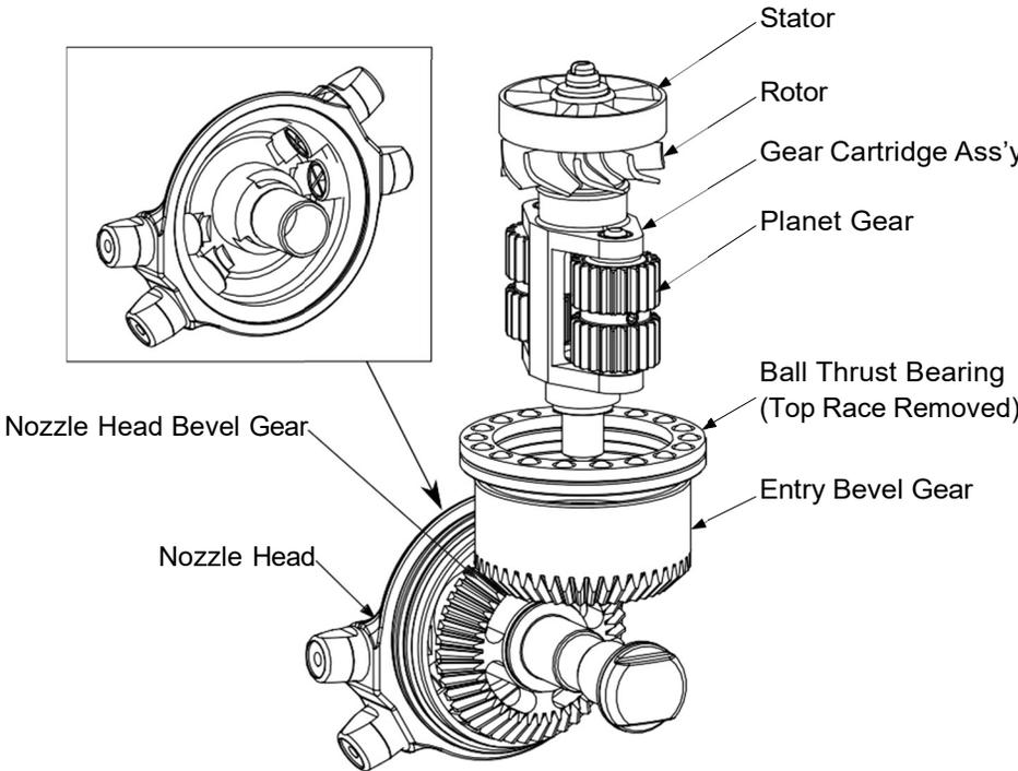
Figure 2: Orbitor 100 tank washing machine with housings removed.
