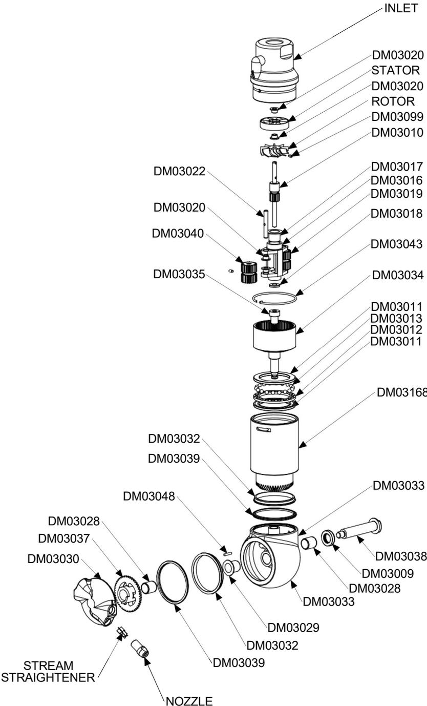
Figure 13: Exploded view of the Orbitor
