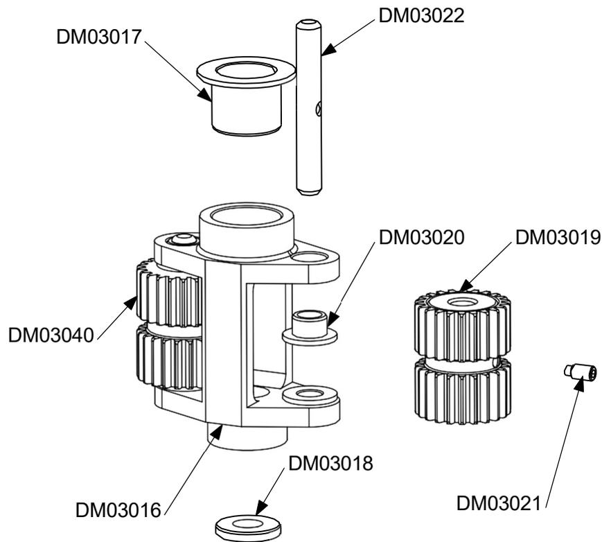
Figure 7: Cartridge subassembly.
