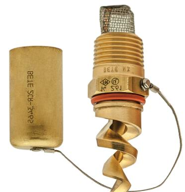
**Fan and Deflected Fan Nozzles:** Fan nozzles are used in water wall fire protection systems because they provide an adequate barrier to shield personnel and equipment against radiant heat, harmful gases, and flames. These nozzles are designed for effective spray impact, and deflected fan nozzles produce an extra-wide spray pattern allowing more water to spray and form a suppression wall.
